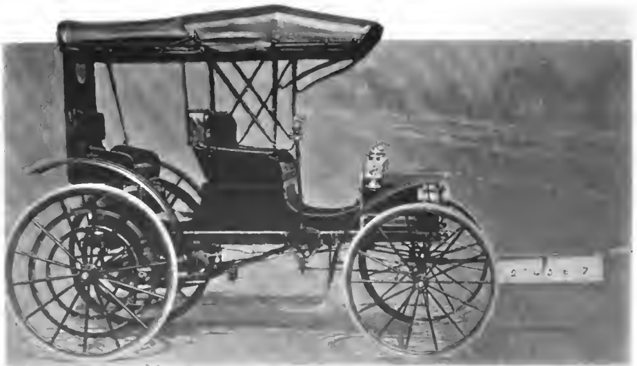
Duryea Car Rigged with a Spring Balance to Measure the Pull Required to Move It.
